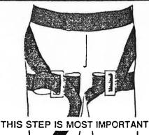
Take the free end of the tape and pass it back under the side of the moveable buckle nearest the loop. This locks the harness. 8
